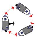
Every year, serious injuries or deaths occur when operators let go of the steering wheel or outboard steering handle while the boat is moving. The steering torque forces the motor to slam left
